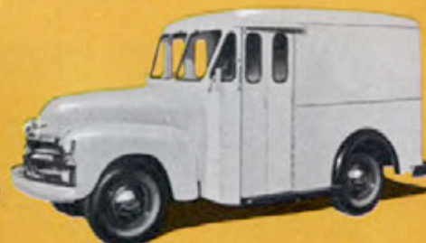
MODEL 3803—CHASSIS AND CAB Accommodates bodies 92" to 116". Weight of body and payload, up to 4900 lbs.
