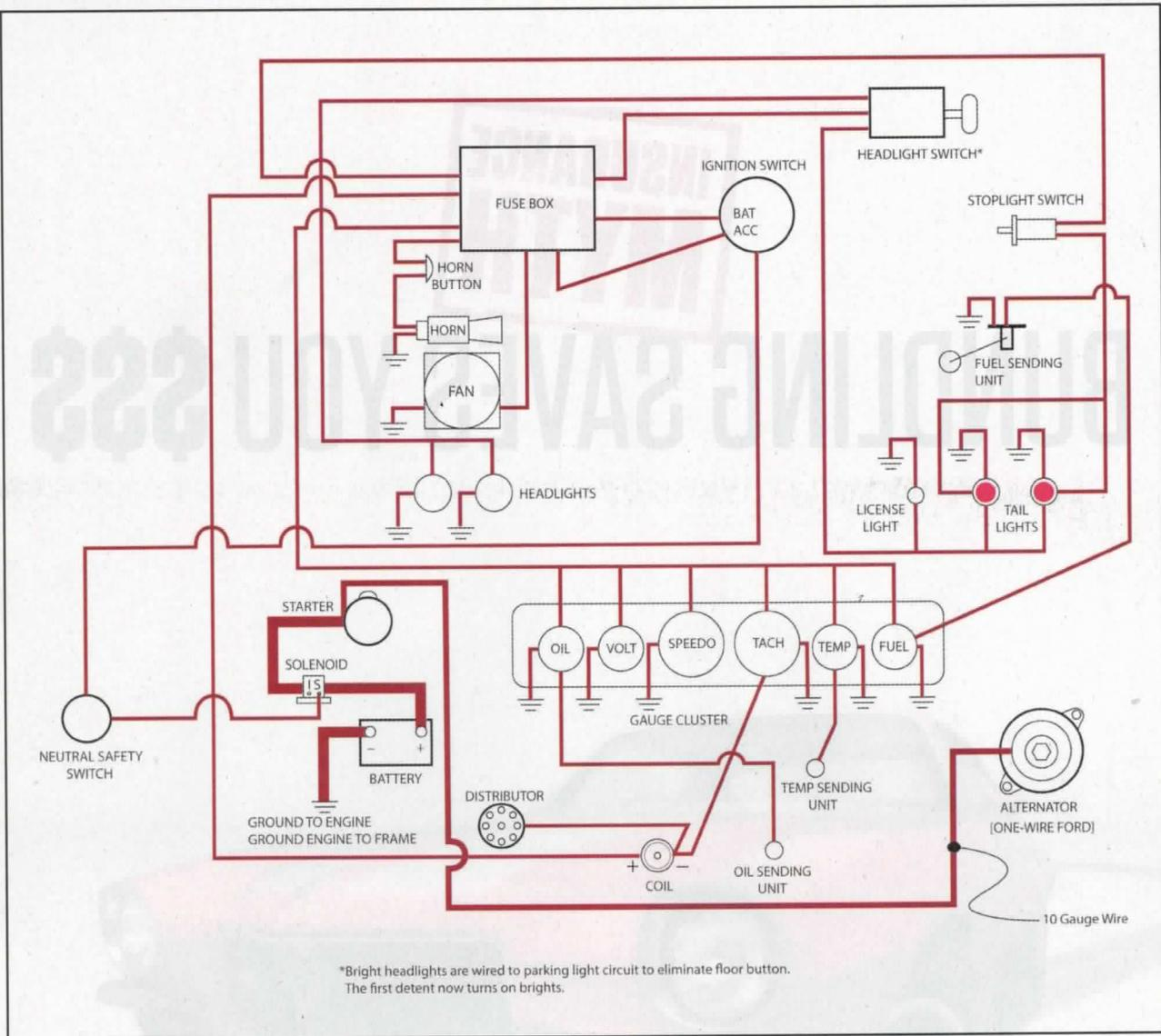
\*Bright headlights are wired to parking light circuit to eliminate floor button. The first detent now turns on brights.
